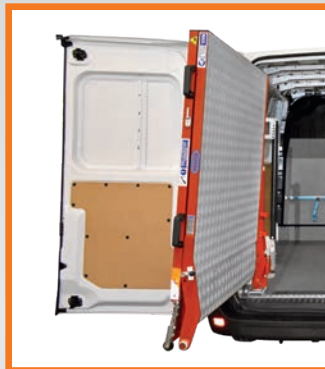
Ramp swung to one side for unrestricted access to the cargo compartment
