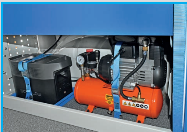
An Ecoflow power station driving a compressor.
