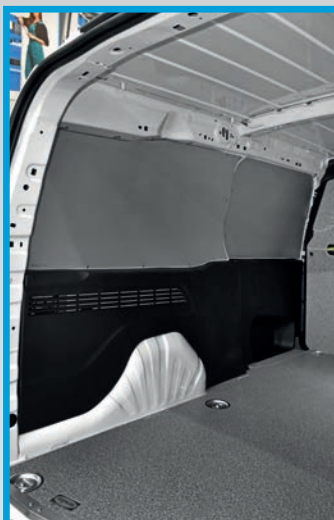
Berlingo/Partner/Combo/Proace City 2018 L2: Floor and bulkhead liners in marble-look birch plywood, bodywork liners in grey prepainted steel sheet
