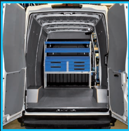
Iveco Daily: racking on the bulkhead only.
