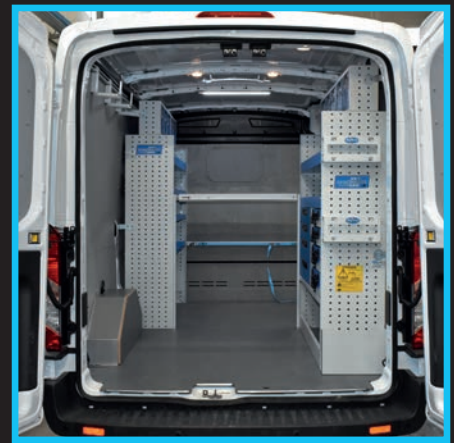
Ford Transit: racking along part of both side walls.
