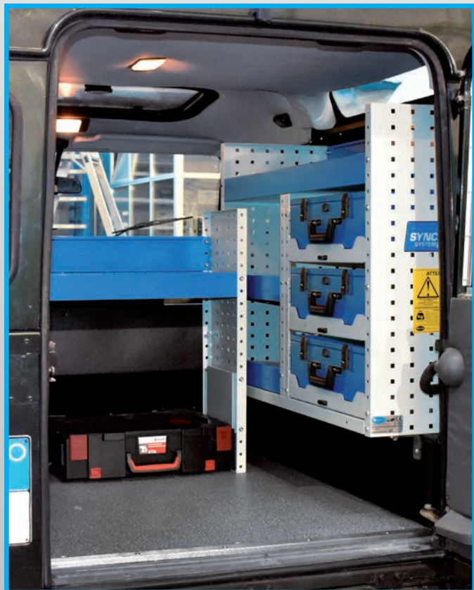
Racking with shelves and drawers in a Land Rover Defender.
