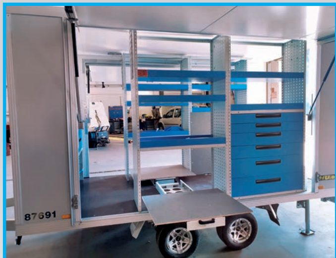
A mobile workshop in an aluminium and fibreglass trailer.
