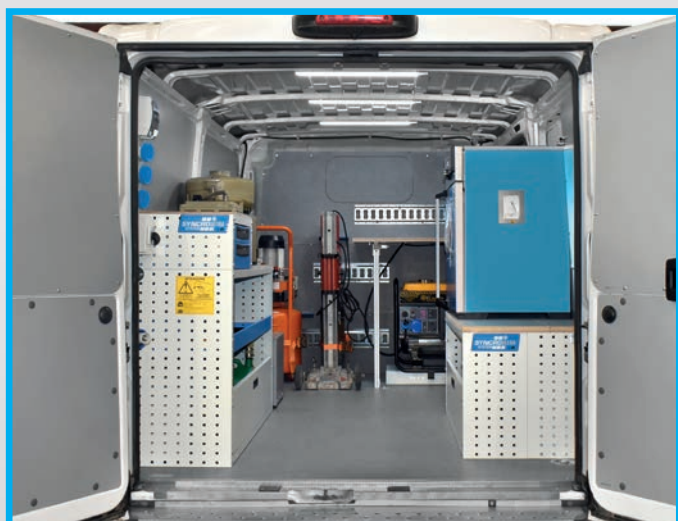
A mobile workshop with compressed air and electrical power supplies and equipment belonging to the customer, installed by Syncro System.
